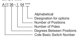
The 1150 series without options if furnished with PC termination, non-shorting and without shaft and panel seals. The standard 10 positions switch is continuous rotation.
